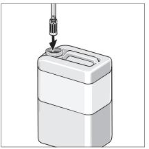
**Step 2** Place the filter end of detergent suction tube into the jug.
